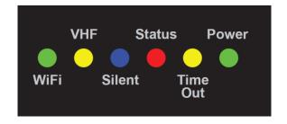
• The VHF LED will only illuminate when you press the Transmit button on the VHF handset. To make sure that the AIT5000's internal splitter is working OK, make a VHF transmission and ensure that the VHF LED illuminates all of the time that you are pressing the VHF Transmit button.
